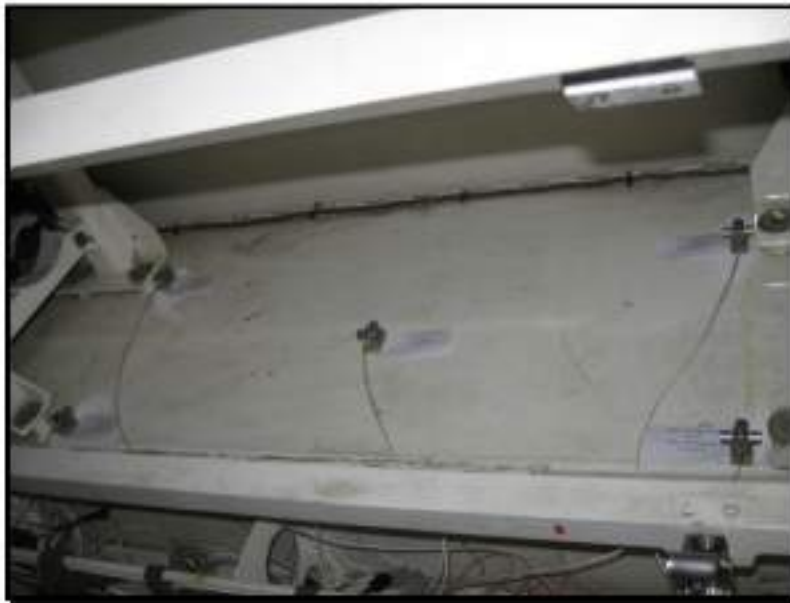
Figure 4. Transducer placement (input to missile rack).
