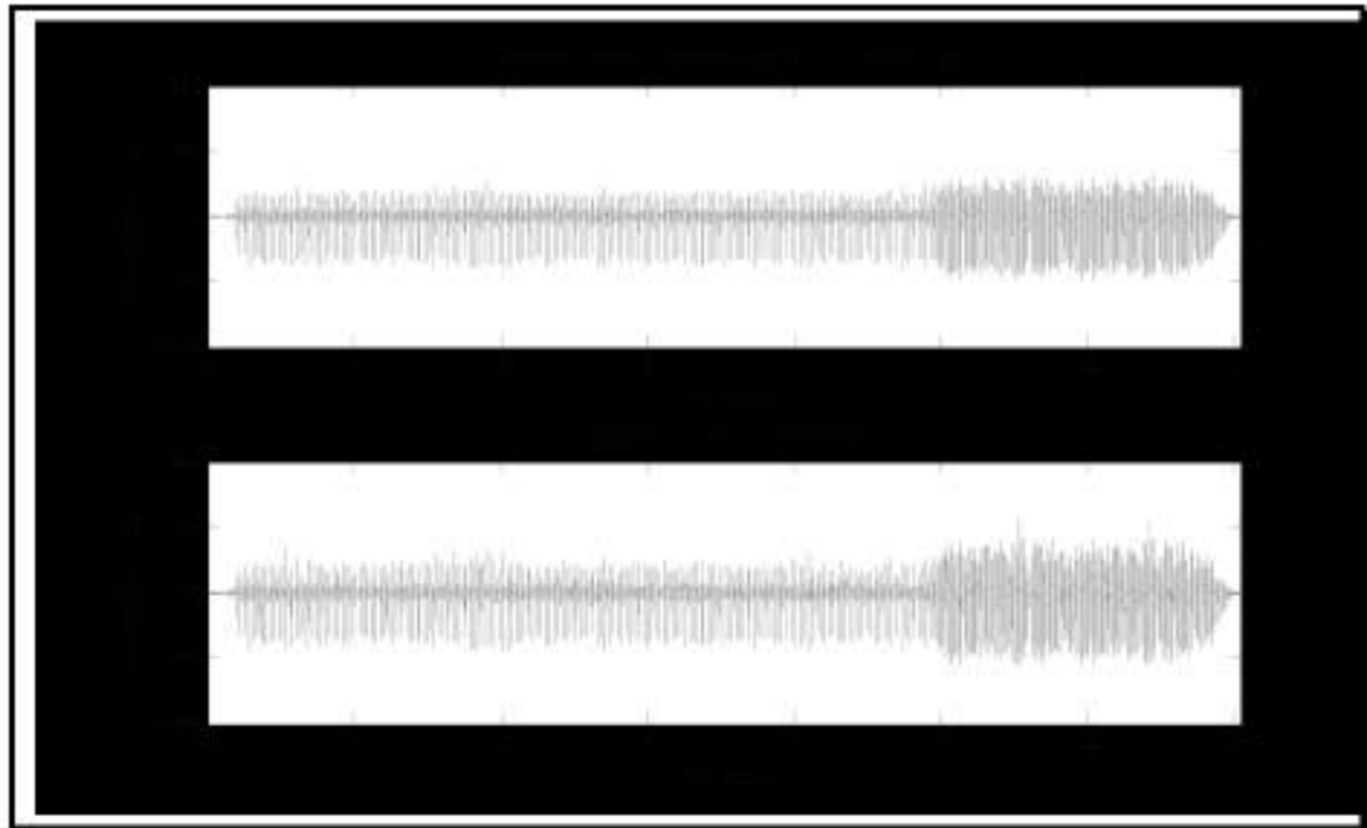
Figure 519.8A-3. Bandlimited (10 Hz to 2000 Hz) and unprocessed TWR test control time traces.
